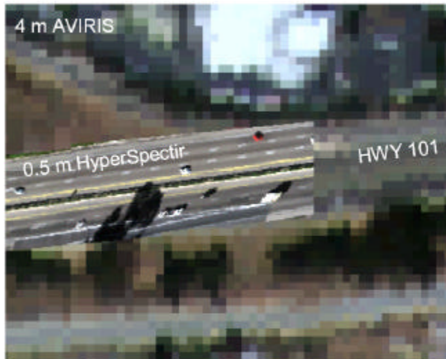
Figure 7: Comparison of spatial detail provided by the AVIRIS and HyperSpecTIR sensor.
