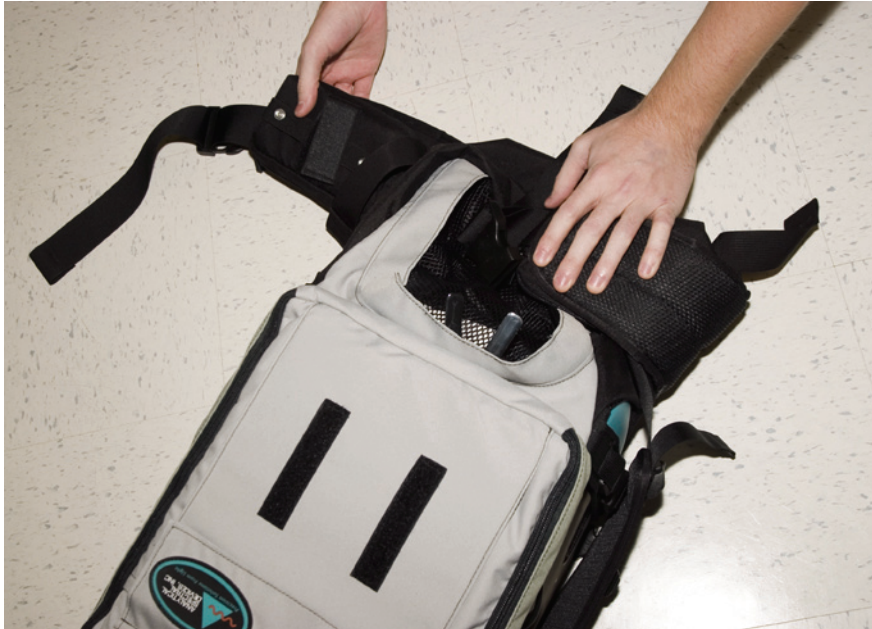
Figure 6-4 Folding the left battery pouches into the Ergonomic Pro-Pack.
