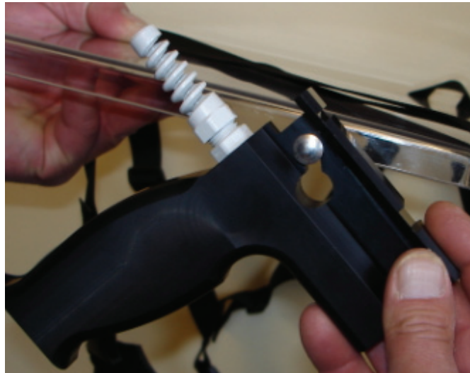
Figure 2-24 Placing the pistol grip onto the pistol grip holder.
