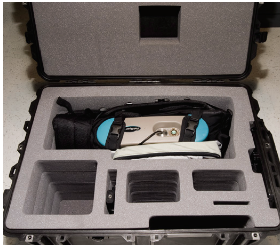
Figure 2-1 FieldSpec spectroradiometer carrying case and foam inserts.
