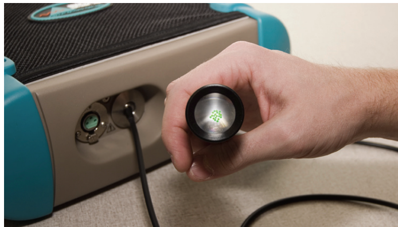
Figure 4-3 Internal spectrometer LED shining to test Fiberoptic cable.
