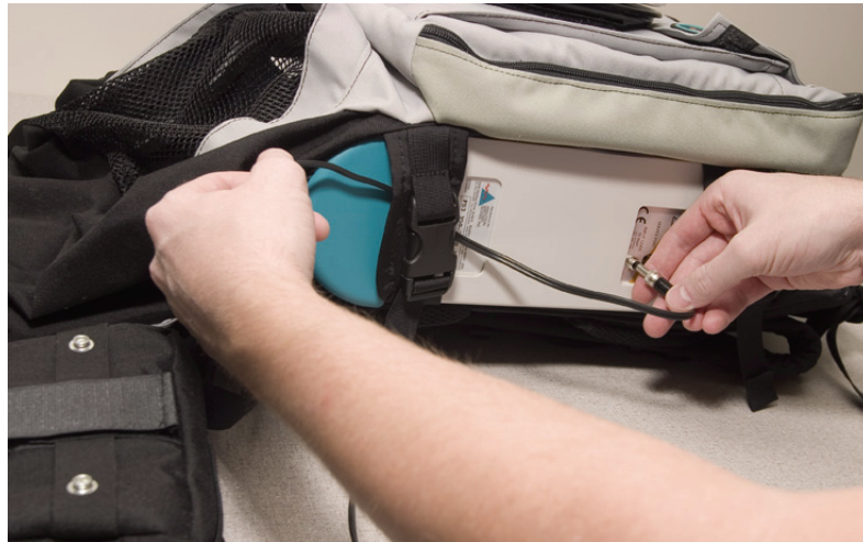
Figure 6-12 Routing the battery cable to the FieldSpec spectroradiometer.
