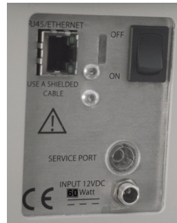
Figure 2-10 FieldSpec spectroradiometer back panel showing Ethernet connection, power switch, and power input jack.
