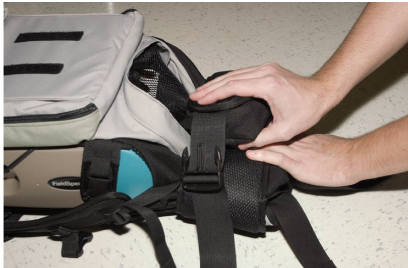
Figure 6-5 Folding the right battery pouches into the Ergonomic Pro-Pack.
