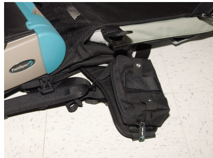
Figure 2-8 Portable battery pack (one on each side of hip belt)
