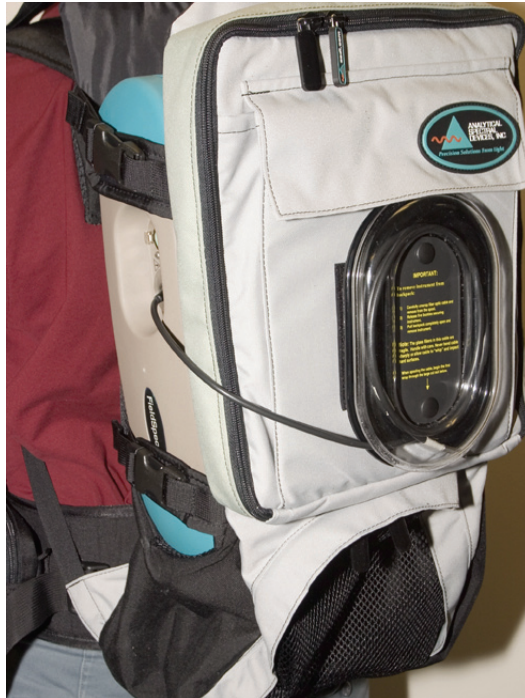
Figure 6-13 Fiber optic cable spool on the outside of the Ergonomic Pro-Pack.
