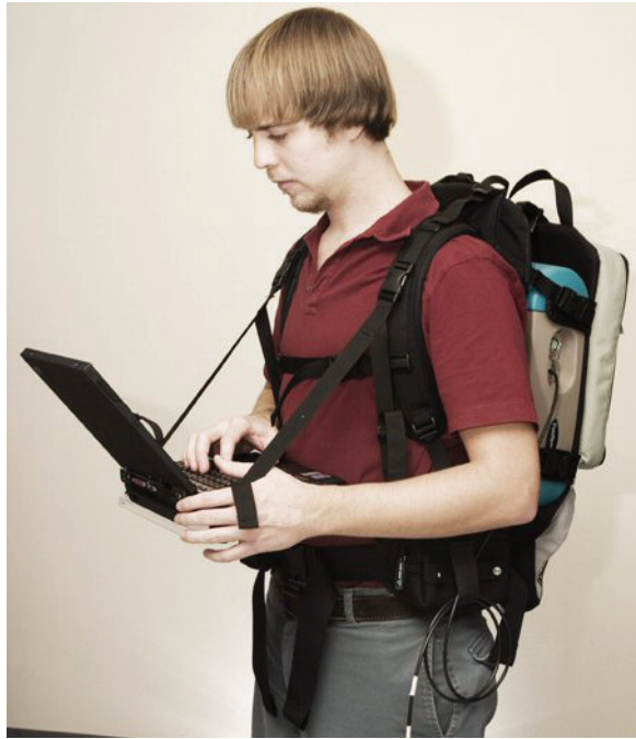
Figure 6-17 FieldSpec spectroradiometer in the Ergonomic Pro-Pack and instrument controller on the laptop carrier.
