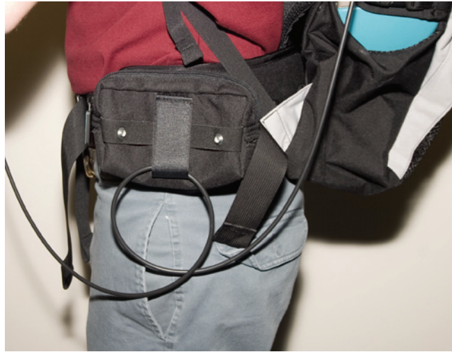
Figure 6-11 Loops for the Fiberoptic cable on the battery pouch of the hip belt.
