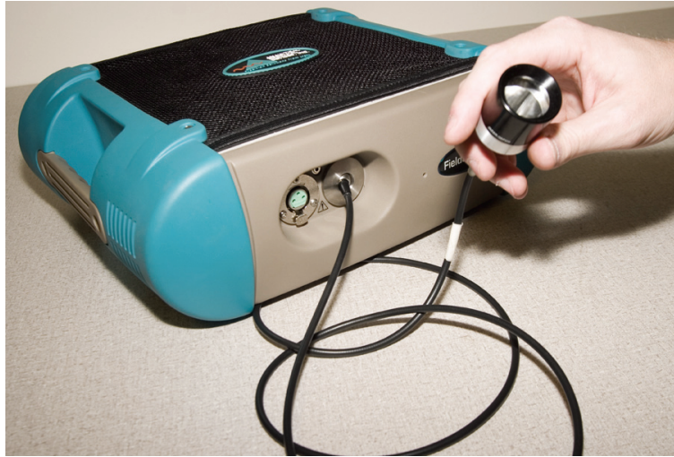
Figure 4-1 Magnifier for testing the Fiberoptic cable.
