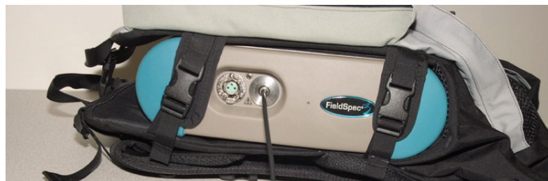
Figure 6-8 Fiberoptic cable routes to either side.
