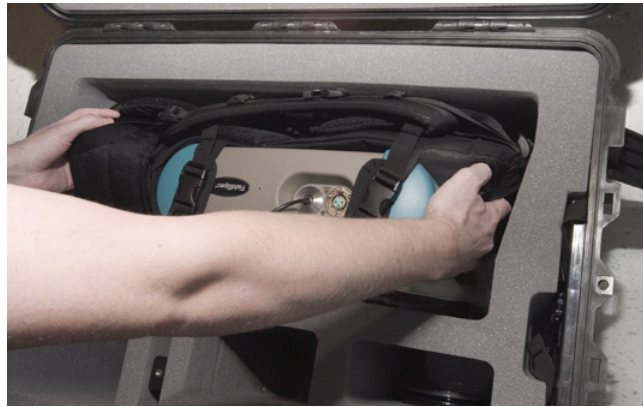
Figure 6-6 Placing the Ergonomic Pro-Pack with FieldSpec spectroradiometer and instrument controller into the shipping case.
