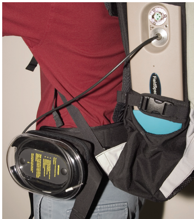
Figure 6-14 Fiber optic cable spool on the battery pouch on the hip belt.
