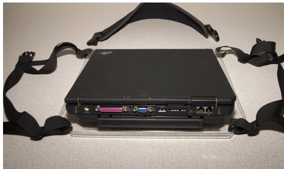
Figure 2-25 The laptop carrier with instrument controller and neck strap.
