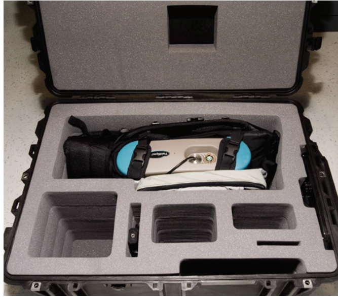
Figure 6-7 Shipping case with Ergonomic Pro-Pack with FieldSpec spectroradiometer and instrument controller.
