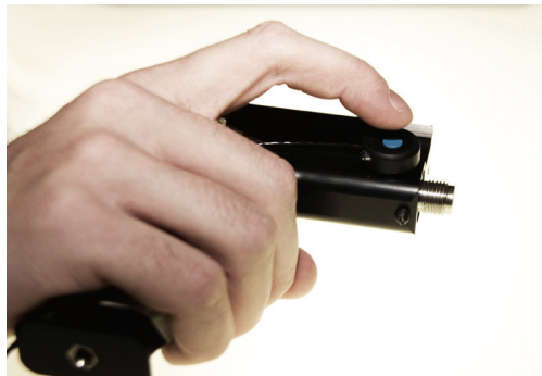
Figure 2-21 The trigger and the Pistol Grip.
