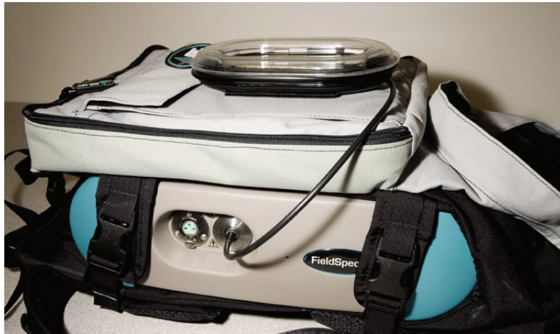
Figure 6-9 Fiberoptic spool on the outside of the Ergonomic Pro-Pack (with velcro).
