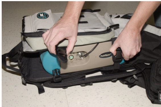
Figure 2-5 Removing the FieldSpec spectroradiometer from the Ergonomic Pro-Pack.
