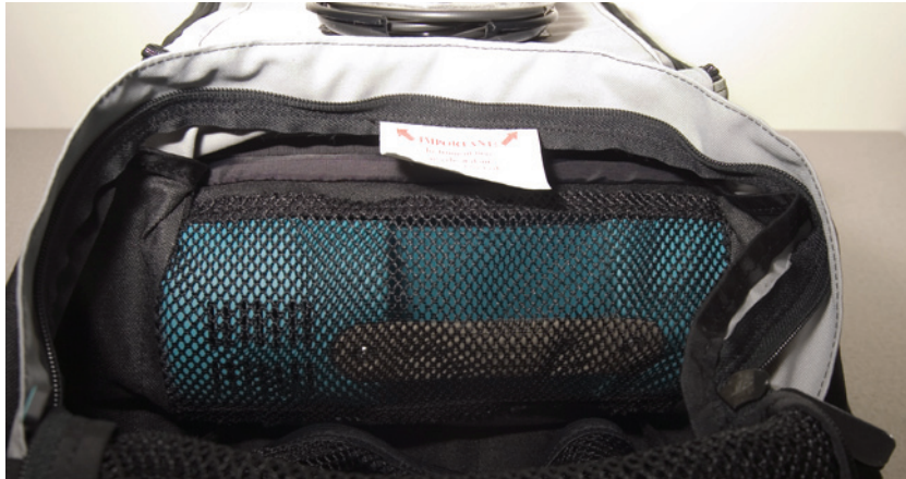
Figure 6-18 Allow for proper ventilation of the FieldSpec spectroradiometer.
