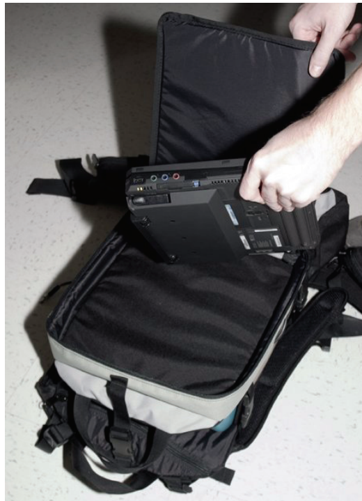
Figure 2-4 Removing the instrument controller from the pack.
