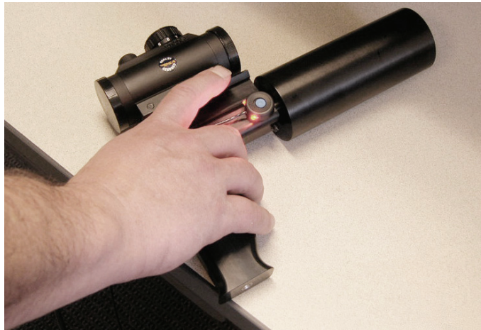
Figure 2-18 Pistol grip with red-dot scope (sold separately), one degree field-of-view (sold separately), and trigger (standard) attached.
