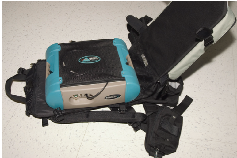
Figure 6-1 The FieldSpec spectroradiometer in the Ergonomic Pro-Pack with cable loosely coiled in the netting.
