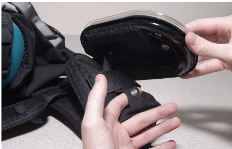
Figure 6-10 Fiberoptic spool and where it attaches with snaps to the battery pouch on the hip belt.
