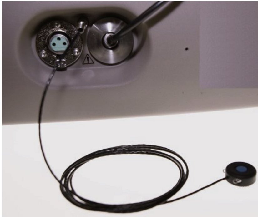
Figure 2-20 External trigger cable plugged into the FieldSpec spectroradiometer.
